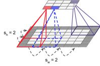
Neuron at row i, column j connects to previous layer's rows  $is_h$  to  $is_h + f_h - 1$  and columns  $js_w$  to  $js_w + f_w - 1$
