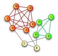
Has a clique of size k = 6, but not of size  $7_{\text{B}}, 7_{\text{B}}$
