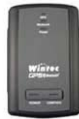
Figure 8 - By functioning as two components, the GPS receiver causes delays in updating the display and consequently inaccurate displayed data [3]
