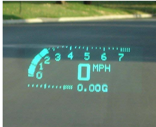
Figure 1 - An example of an HUD used to display the speed of a car to its driver [1]
