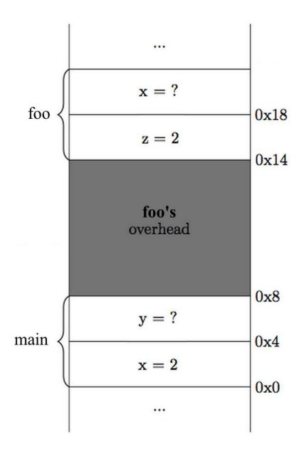
Because foo is the top plate on the stack, we only see its local variables, thus there is no problem with different variables with identical names as long as they are used in a different method.
