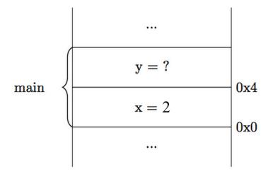
But in order to get a value for y, we must first execute the method foo. In order to prepare for foo to be called, main must place some overhead on the stack, then it must push any parameters necessary for foo on the stack. And so, when foo is called, it begins execution with the following execution stack.
