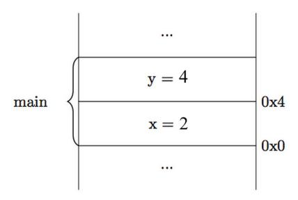
Where the 4 was the return value of the function call (foo). At this point the execution of our program is finished. Main will pop the rest of its stack frame, signaling the end of execution.
