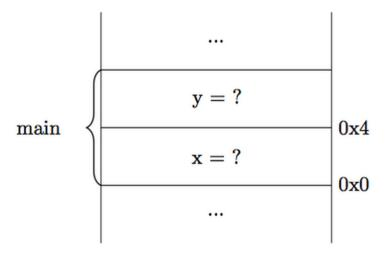
This **stack diagram** is a representation of memory in a computer. Memory is laid out logically starting at address 0x0 and ending with address 0xffffffff (notice how the numbers get *larger* as the stack grows.)
