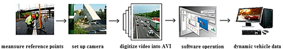
Fig. 2 Traffic data collection and extraction using video-capture techniques
