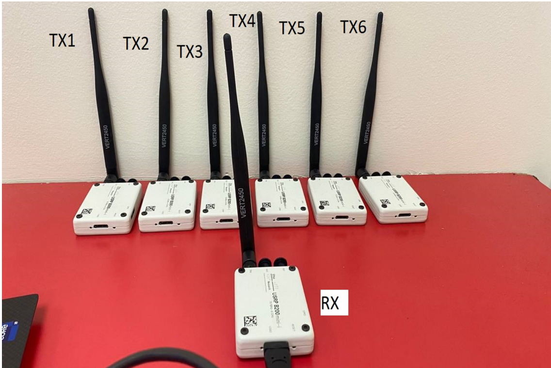
Figure 6.1: Testbed: One receiver and six transmitters
