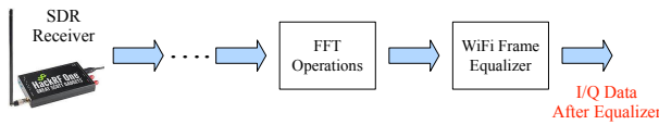
Figure 2: I/Q data collection in GNU Radio at the Receiver. We collected I/Q data after WiFi Frame Equalizer.
