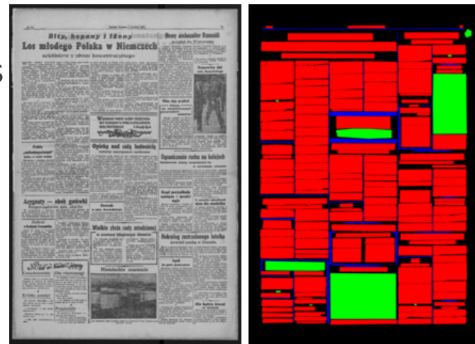
Figure 4. Example of image (left) and ground-truth (right) from ENP dataset. In the ground-truth, each color represents the following components: (1) black: background, (2) red: text, (3) green: figure, (4) blue: line-separator, and (5) yellow: table.
