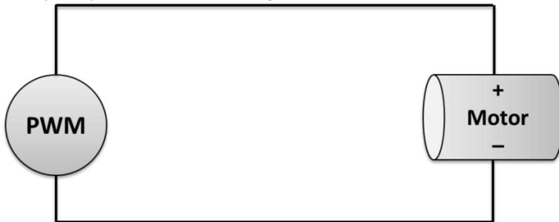
Figure 2: The PWM signal creates a certain duty cycle which will provide an "average" voltage to the motor. This average voltage is proportional to the motor's output torque.
