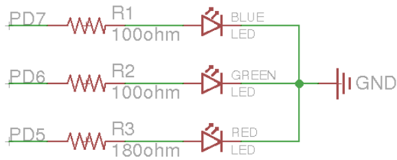
Figure 1: Schematic diagram for the LED connections.
