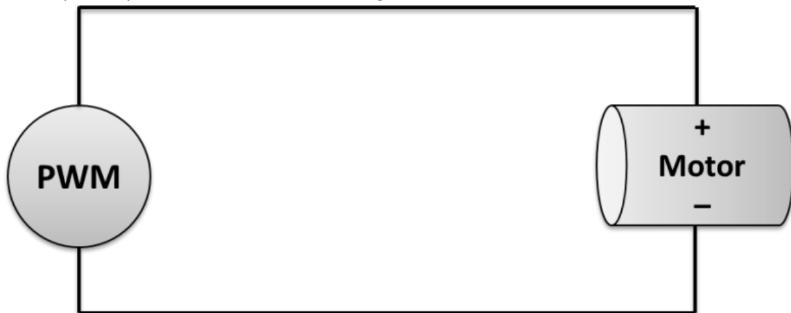
Figure 2: The PWM signal creates a certain duty cycle which will provide an "average" voltage to the motor. This average voltage is proportional to the motor's output torque.
