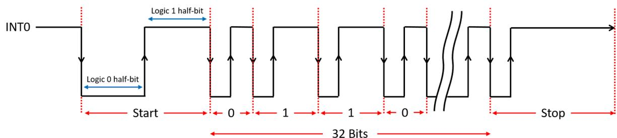
Figure 4: IR receiver signal showing all bits
