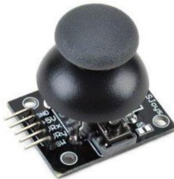
Figure 1: Analog Joystick Module
