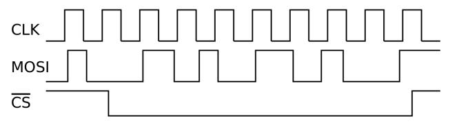
**b).** (10 pts) In the above signal, what is the data stream (bit values) processed by the slave device if it is configured for data to be valid on the rising edge? What about for falling edge? Note that the CS ("not CS") line means the device is active low, in other words it is selected when the line is low.
