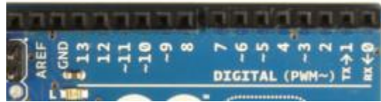
Figure 4: Digital Pins on Arduino Uno
