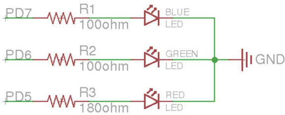
Figure 1: Schematic diagram for the LED connections.
