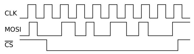
**b).** (5 pts) In the above signal, what is the data stream (bit values) processed by the slave device if it is configured for data to be valid on the rising edge? What about for falling edge? Note that the CS ("not CS") line means the device is active low, in other words it is selected when the line is low.
