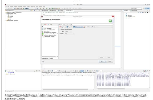
23. Display Hello World Output on SDK built-in console window
