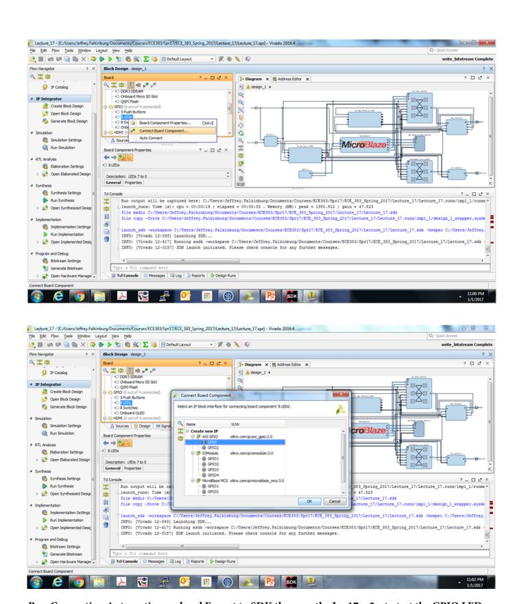
Run Connection Automation and Export to SDK then use the Lec17\_v2.c to test the GPIO LEDs
