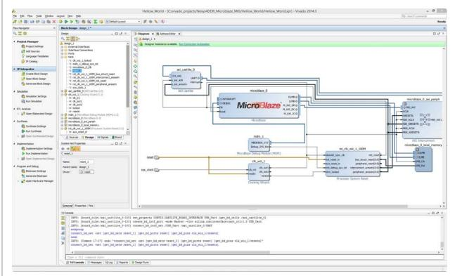
7. Adding and Customizing Memory Interface Generator IP Block
