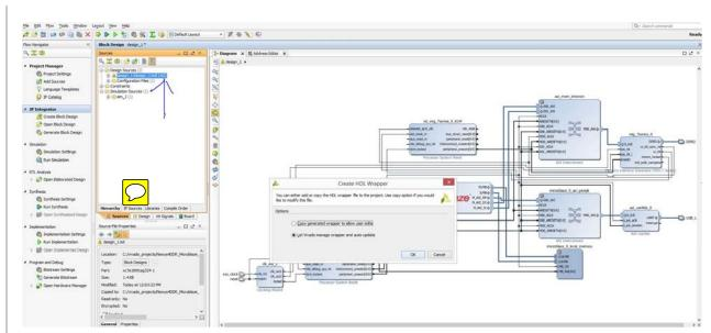
12.2) A system wrapper file will be generated and a message will be displayed in the tcl console informing us that the *wrapper.v* file has been generated.
