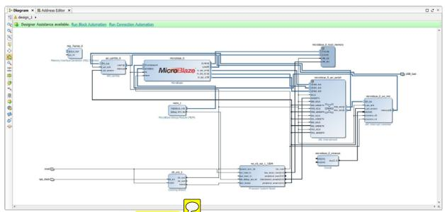
7.2) After adding the MIG IP block, double click on the block to **Run Block Automation**.
