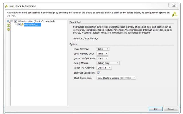
3.4) Running the block automation will auto-generate a set of additional IP blocks which will be added to our hardware design automatically based on the options selected in the previous step. **Do not click on Run Connection Automation yet.** Note: You can right click and select Regenerate Layout at any time to clean up the layout, potentially making it easier to read.
