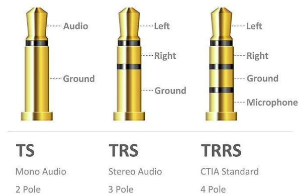
Figure 2: Typical Stereo Jack pinout
