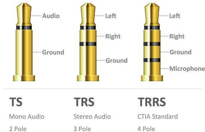
Figure 2: Typical Stereo Jack pinout
