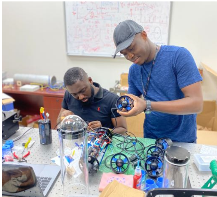
FIGURE 3.1: Assembly of the BlueROV2
