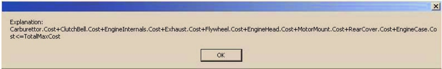
Fig. 8. An explanation showing the cost constraint that the Carb1.0.iam assembly has violated.
