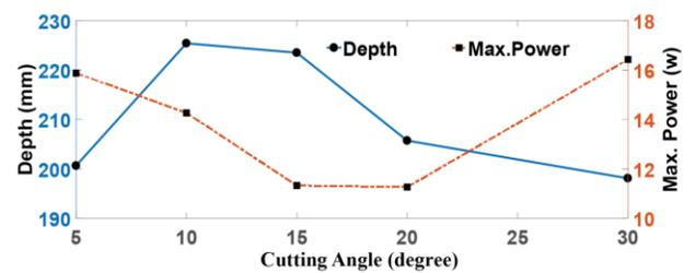
Fig. 8: Digging performance of different cutting bits.
