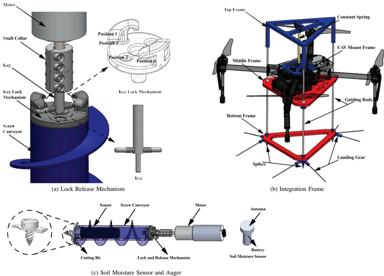
Fig. 3: Mechanical system details.
