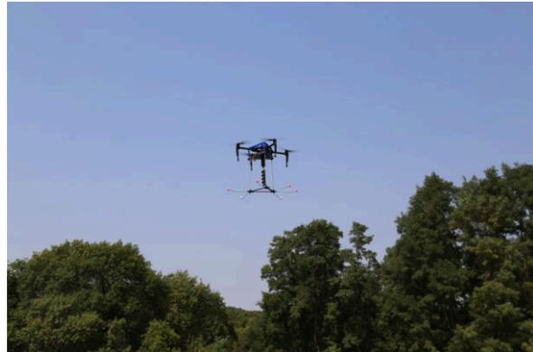
Fig. 1: The unmanned aerial auger in flight.
