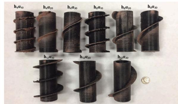
Fig. 7: Screw conveyors.
