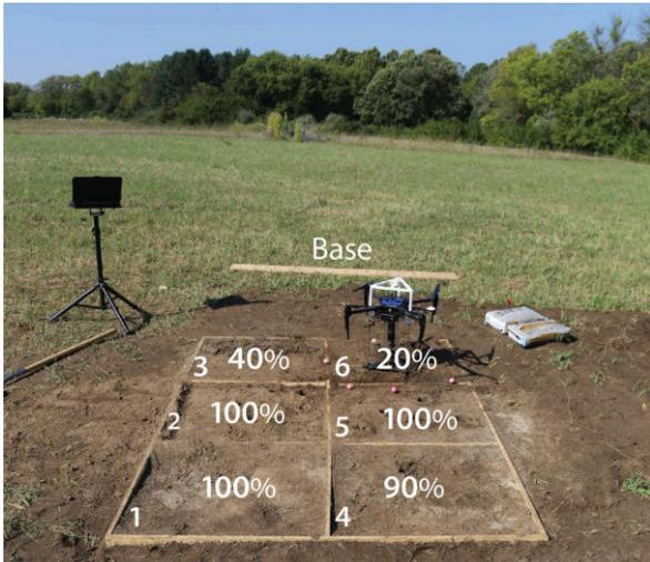
Fig. 10: Field testbed with six soil types (success percentage).
