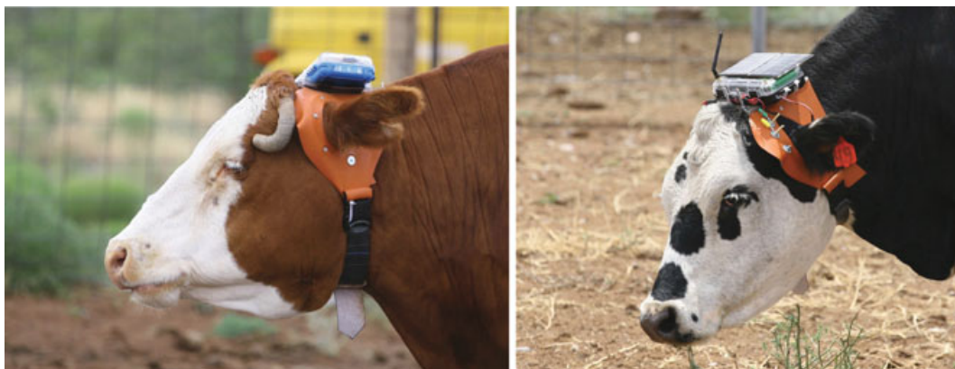
Figure 4. The sensor box is mounted to the head of the cow with a custom-fitted apparatus made of fabric and plastic. The apparatus is designed to use the cow's ears to keep the box in an upright position, as shown in this figure.
