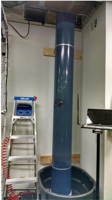
Fig. 4. 10ft vertical water column for in-water lab testing
