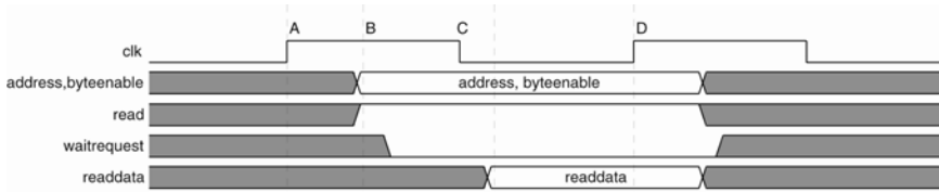
Figure 14: Fundamental Master Read Transfer with No Wait-States
