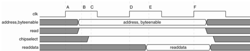
Figure 5: Slave Read Transfer with One Fixed Wait-State
