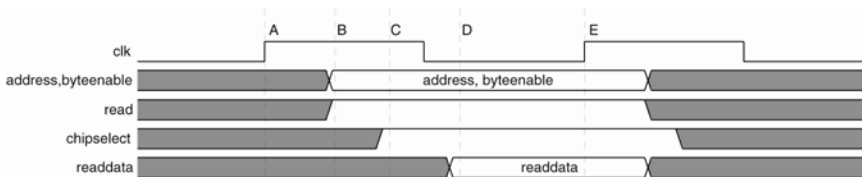
Figure 4: Fundamental Slave Read Transfer
