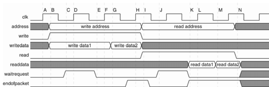
Figure 23: Master Read and Write Transfers with Flow Control
