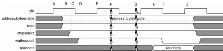
Figure 7: Slave Read Transfer with Variable Wait-States
