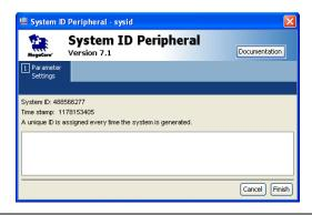
3. Click **Finish**. You return to the SOPC Builder **System Contents** tab, and an instance of the system ID peripheral named **sysid** now appears in the table of available components.
