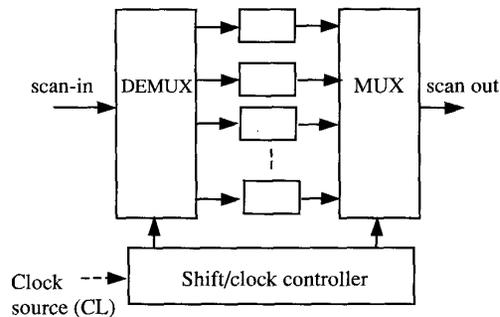
Figure 1b: Fully parallel scan-path
