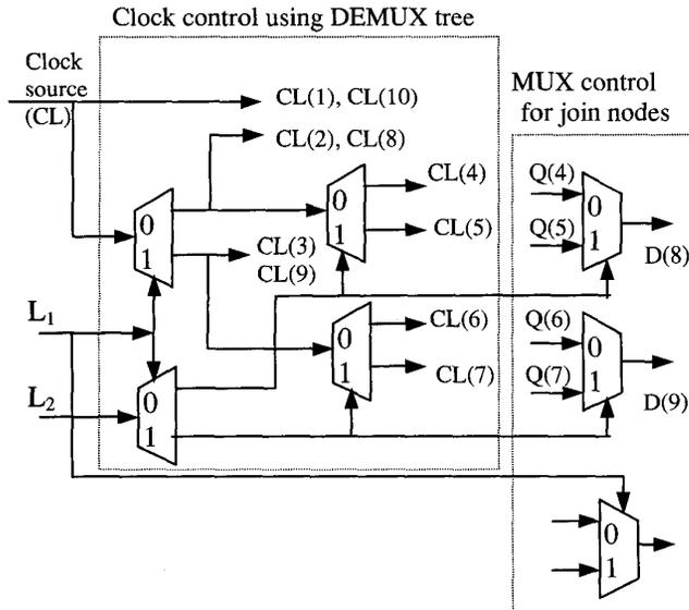
Figure 4: A hierarchical clock gating logic for DTS(2)
