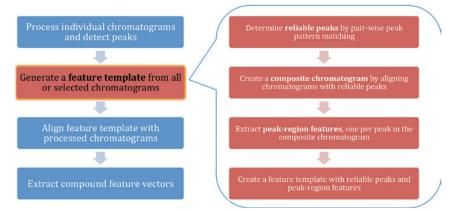
Figure 1. Automated Investigator Workflow. The workflow detects and aligns all compounds from multiple chromatograms, and extracts feature vectors for untarged cross-sample analyses.
