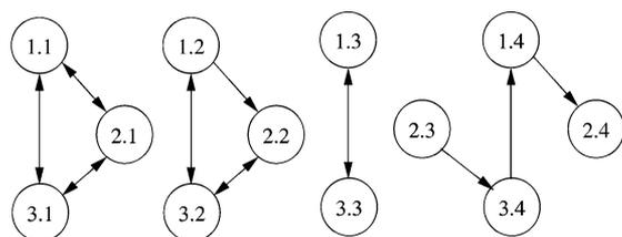
**Figure 3.** Example pairwise matchings, shown by arrows, between four peak features in each of three chromatographic patterns — Peaks 1.1–1.4 in Pattern 1, Peaks 2.1–2.4 in Pattern 2, and Peaks 3.1–3.4 in Pattern 3.
