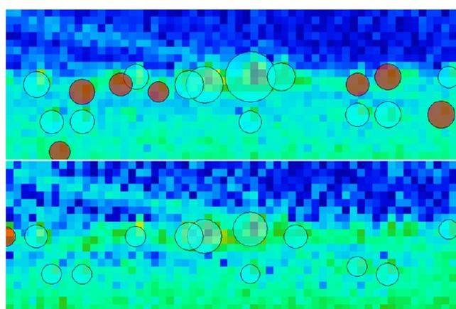
**Figure 2.** Small subregions of two chromatograms from different bio-oil samples. The data points in this figure are shown as rectangles to clearly illustrate the granularity of the modulator and detector sampling. The peaks marked by cyan-colored bubbles are definitively matched in each direction, but the peaks marked by red-colored bubbles are not definitively matched.
