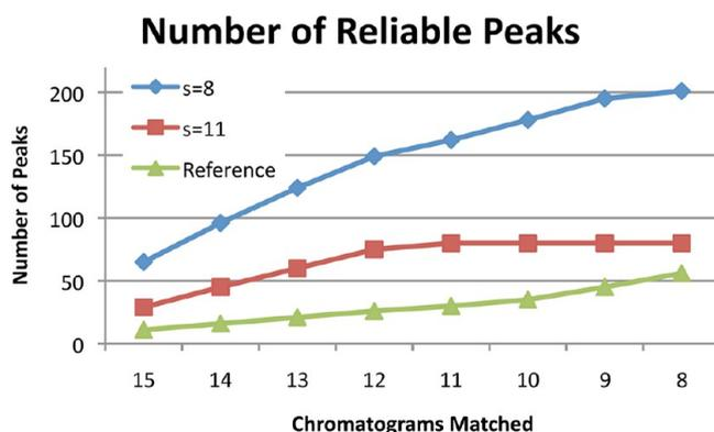
**Figure 8.** Graph shows the number of conflict-free, reliable peaks as a function of the number of chromatograms matched for (a) CCM with  $s = 8$ , (b) CCM with  $s_{15} = 11$ , and (c) using a reference chromatogram. At all levels of reliability, CCM yields a greater number of reliable peaks than does matching with a reference chromatogram.
