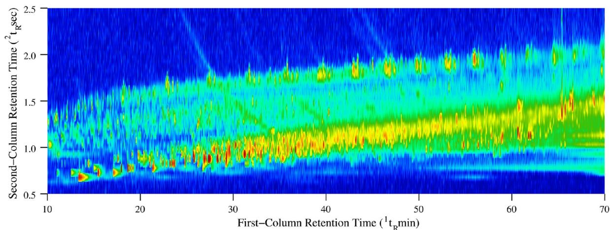
**Figure 1.** Pseudocolored image of the total intensity count (TIC) for a GCxGC-MS chromatogram from a complex bio-oil. Each compound produces a two-dimensional peak in the data array output by the detector. Only a subregion is shown.
