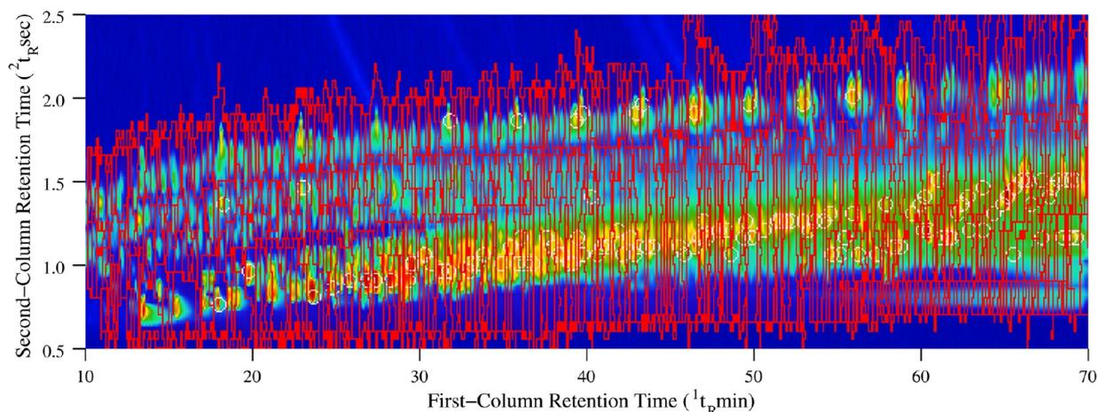
**Figure 9.** Pseudocolored image of the total intensity count (TIC) for the composite chromatogram from fifteen aligned chromatograms. The overlay shows the reliable peaks (with white circles) and the regions of the detected peaks (with red dotted outlines).
