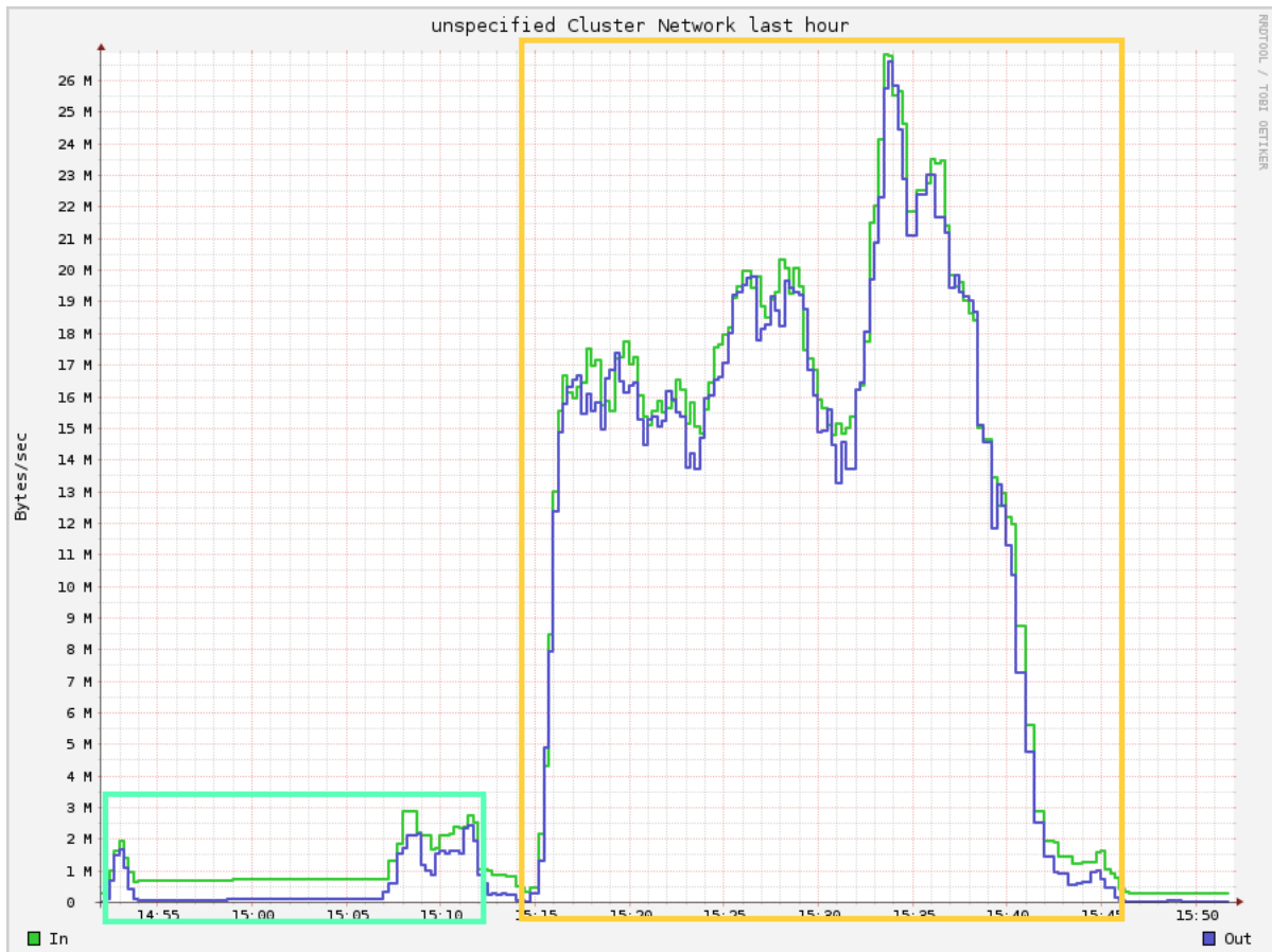
Figure 5.12: Network utilization. Note the minimal use by the MapFile store (left) compared to the HBase store (right).
