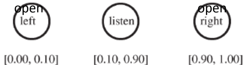
Fig. 10. The optimal situation-action mapping for t = 1 for the tiger problem shows that each of the three actions is optimal for some belief state.
