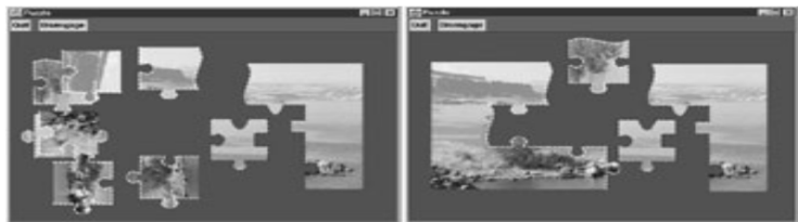
Figure 1: ROAMINGJIGSAW. When a player is disconnected (left), only the pieces previously selected can be assembled. Upon reconnection (right), the assemblies made meanwhile by other players become visible in the player's workspace.
