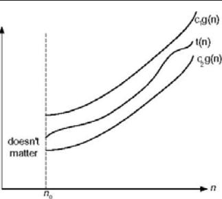
Figure 2.3 Big-theta notation:  $t(n) \in \Theta(g(n))$
