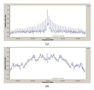
Fig. 10. The Spectrum of Received Signal in Underground to Aboveground Communication: (a) Transmitter Muted, (b) BPSK Signal Transmitted.
