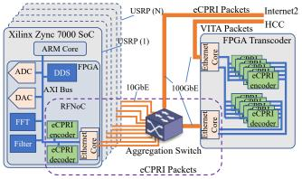
Fig. 5. The Schematic of Fronthaul Logical for eCPRI.
