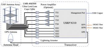
Fig. 2. Software Defined Distribution Unit Schematic.
