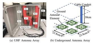
Fig. 3. UHF Antenna Array: 2x2 Uniform Rectangular Array.
