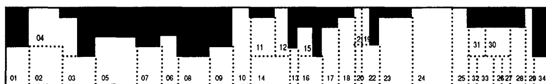
Figure 3. Optimal solution of the ship loading problem with a limit of eight people (fixed duration).
