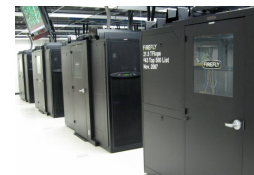
Figure: 2007: Firefly built; 1,151 nodes (280 AMD Quad core, 871 dual core Opteron), 43rd fastest super computer at the time.
