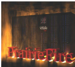
Figure: PrairieFire is a 98-node Beowulf cluster, originally constructed in 2002. It originally scored an HPL benchmark number of 442.50 GFlops, which was then the 107th most powerful supercomputer in the world, according to the TOP500 supercomputer list. See http://rcf.unl.edu/prairiefire/index.php
