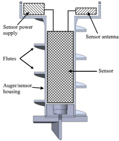
Fig. 2: Auger with internal sensor
