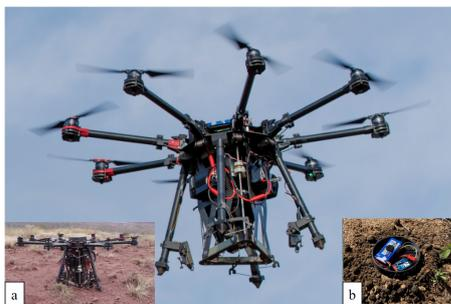
Fig. 1: Sensor emplacement system.
