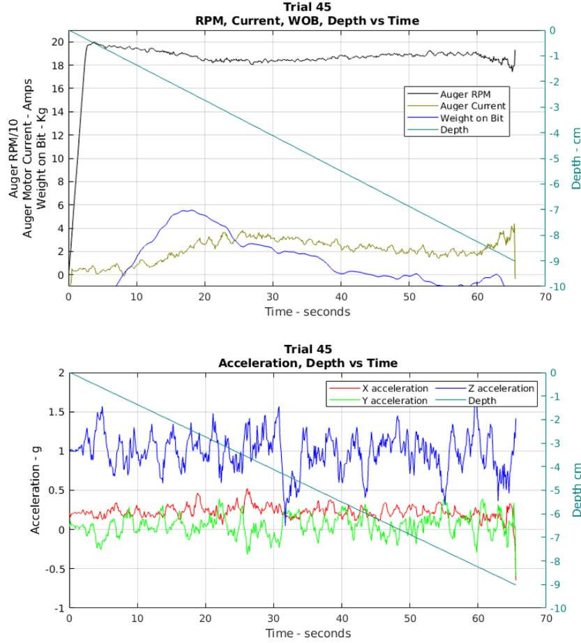
Fig.8: Example of parameters gathered during system trials. The top graph shows auger RPM, motor current, weight on bit, and depth over time. The bottom graph show accelerations in the x, y, and z axes and depth over time
