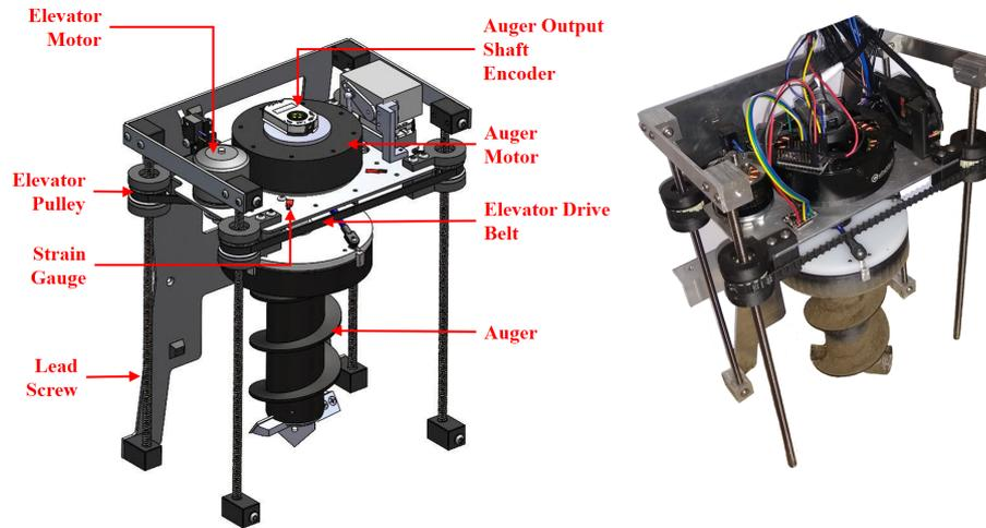
Fig. 3: Emplacement mechanism: model (left) and system (right)
