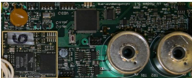
Figure 3-9: Picture of the acoustic modem
