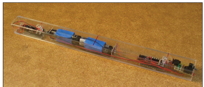
Figure 12. The passive bar with embedded IR LEDs and batteries.
