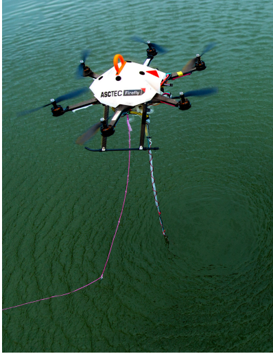
Figure 1: UAV-system with a passive cable and sensors for measuring water properties at precise depths.
