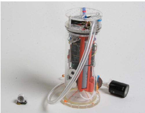
Fig. 3: The receiver and transmitter of AquaOptical can be seen on the left. A sensor node with the short range receiver and transmitter integrated in the top cap is displayed on the right.
