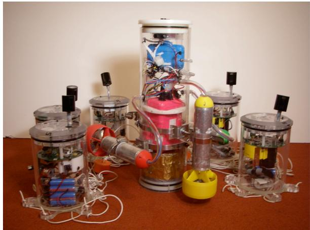
Fig. 2. A picture of AMOUR and some sensor nodes.
