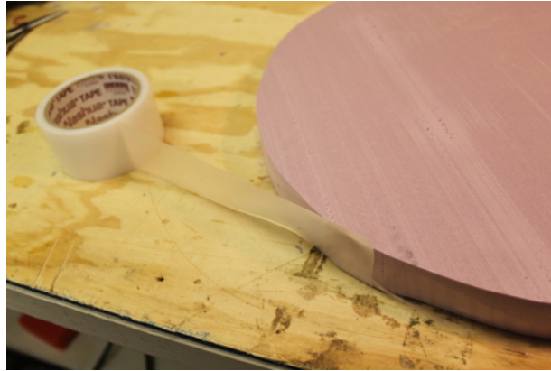
Figure 4: Taping the plastic disk to the hovercraft base.
