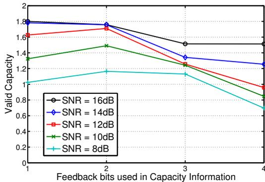
Fig. 7. Valid capacity versus Bit used in Capacity Information in different SNR .
