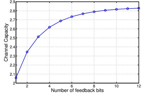
Fig. 5. Capacity of MIMO radio link under different numbers of feedback bits.
