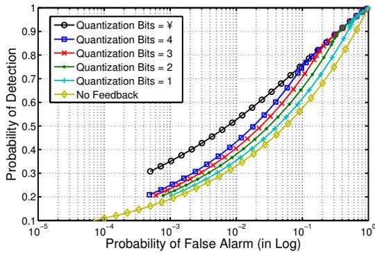
Fig. 2. Probability of detection and Probability of false alarm curves for different feedback bits.
