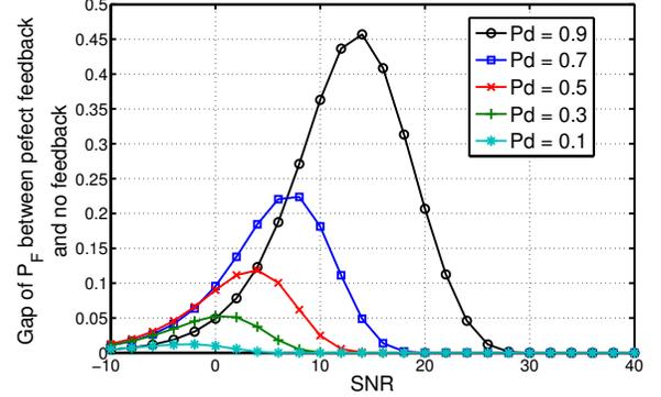
Fig. 3. Gap of  $P_F$  between Perfect feedback and No feedback in different SNRs.
