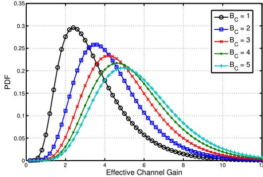
Fig. 4. PDF of the effective channel gain for different feedback bits.
