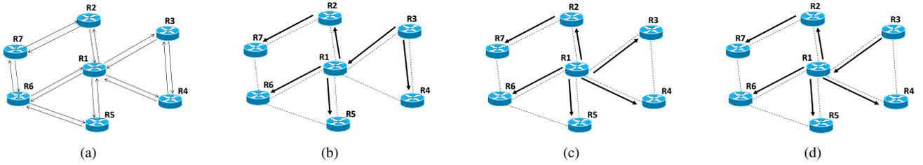
Fig. 2. a) Example of a network graph with OSPF weights. b) SPT computed by  $R3$ ,  $SPT(R3)$ . c) SPT computed by  $R1$ ,  $SPT(R1)$ . d) EAR algorithm performed by  $R3$  if  $R1$  is the exporter router,  $MPT(R3, R1)$ .
