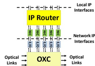
Fig. 1. Architecture of an IP-over-WDM node.
