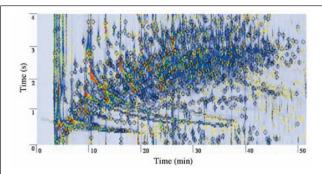
**Figure 3.** GC×GC–MS chromatogram for standard-roast Colombian coffee. Circles indicate the retention times of 1652 peaks. Black circles indicate the subset of 891 reliable peaks that were consistently matched for a set of three chromatograms (including this chromatogram and chromatograms of standard-roast Brazilian and Guatemalan coffees), and yellow circles indicate unreliable peaks that were not matched consistently for the set.
