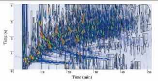
**Figure 5.** Mesh panels (shown as black polygons) for analysis of the set of three chromatograms from standard-roast coffee overlaid on the cumulative chromatogram. There are 34 meshes covering the chromatographic features divided into 1109 panels. The consensus template also contains the reliable peaks shown in Figure 3.
