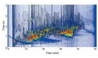
Figure 7. Cumulative chromatogram for a set of six Juniper samples with a template of reliable peaks indicated by yellow circles and mesh panels indicated by black outlines.
