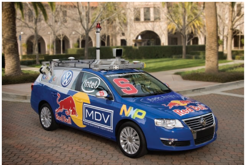
"Junior," a driverless 2006 Volkswagen Passat modified by the Stanford Racing Team for the 2007 Urban Challenge.
