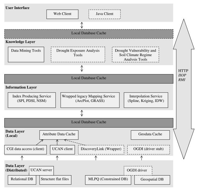
Figure 3. The four-layer distributed GDSS software architecture developed for the NADSS Project.
