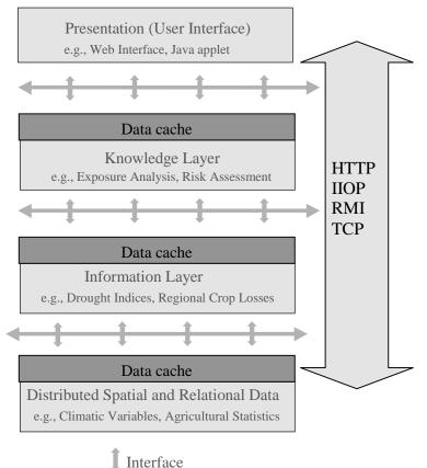
Figure 1. A four-layer software architecture for distributed geospatial decision support systems.
