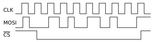
b) (5pts). In the above signal, what is the data stream (bit values) processed by the slave device if it is configured for data to be valid on the rising edge? What about for falling edge? Note that the  $\overline{CS}$  ("not CS") line means the device is active low, in other words it is selected when the line is low.
